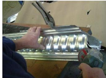
2. Clamp to hold in place prior to Cutting, cut to the outer side of line.
